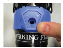
**STEP 4** - Move the shaper into the STRAIGHT STREAM position. Wrap the new tactile Indicator around the Stream Shaper with the tab on top. The 3 tabs on the inside of the indicator will snap into the 3 grooves around the shaper. Close the tab to align the hole in the indicator tab with the threaded hole on the top of the Stream Shaper.
