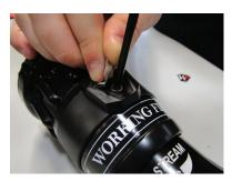
**STEP 1** - Remove the label from the Tactile Indicator, then remove the screw using a 5/32" hex key.
