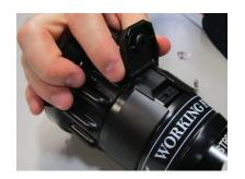
**STEP 2** - Lift the rear edge of the indicator tab so it hinges upward.
