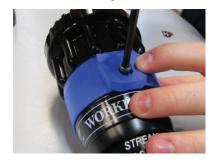
**STEP 5** - Apply Loctite 271 sparingly to the screw threads and install until snug using a 5/32" hex key.
