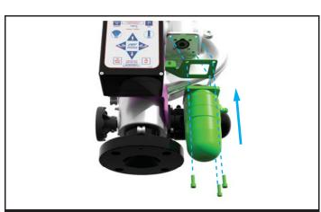
STEP 8 - Align Vertical Motor Housing & Y2131 Bracket. Leave the motor mounting screws slightly loose until all items have been installed then tighten all screws. Tighten 3X Socket Head Screw(s)
