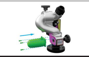
STEP 7 - Align Horizontal Motor Housing & Y2130 Bracket. Leave the motor mounting screws slightly loose until all items have been installed then tighten all screws. Tighten 3X Socket Head Screw(s)
