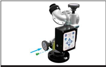
STEP 9 - Lift Control Box And Tighten 1X Stop Bolt Or 1X Socket Head Screw(s). If a set screw was originally installed in this location it will be replaced by the 3/8" socket head screw included in the kit.
