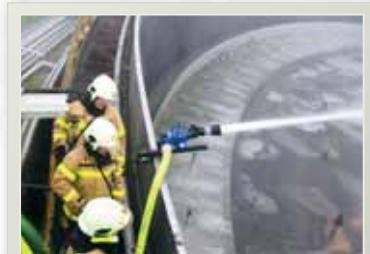
KLEMMT SICH SICHER AN LIPPEN VON MINERALÖLBEHÄLTERN
