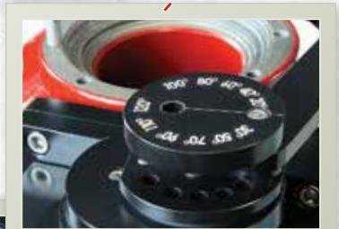
Adjustments from 0-120 degrees in 10 degree increments
