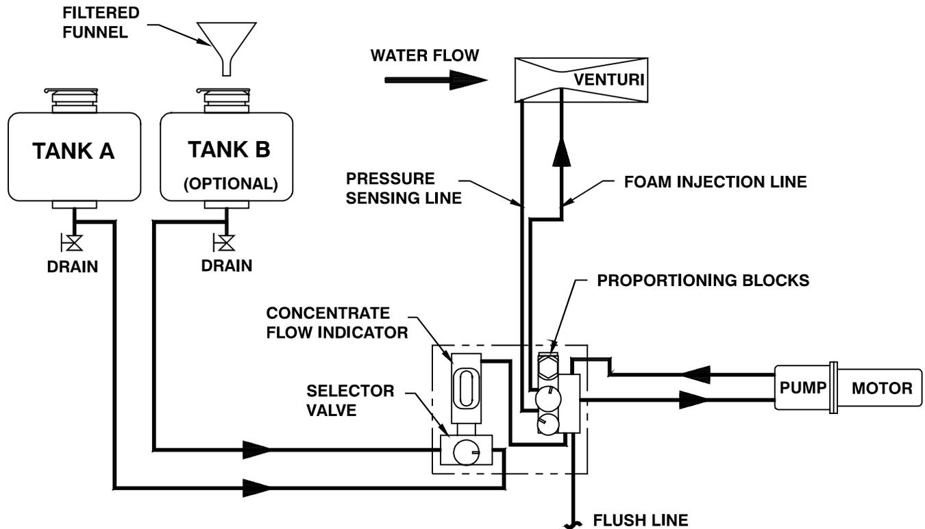
**FIGURE 2 PANEL MOUNT PRO/PORTIONER SYSTEM DIAGRAM**
