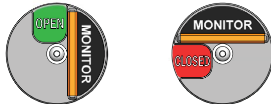
Figure 5.1.2: Monitor valve position indicator (orange flag)
