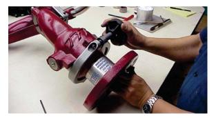
Remove knob assembly. Remove cotter pin from end of locking nut. Remove locking nut, castle nut, washer and knob.
