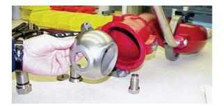
9) Grasp ball with hex hole on the bottom and circular opening on the right.
