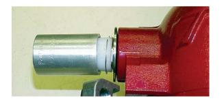
Install Smalley Ring to retain Belleville spring on trunnion.
