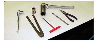
Tools used for ball valve assembly:
