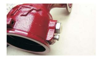
19) Install stationary trunnion into bell section with red Loctite. Turn trunnion in until tight making sure that it engages the threads in the ball.
