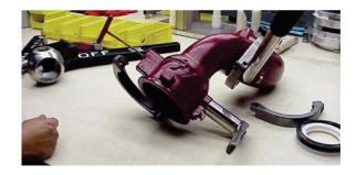
5) Using 1-1/8" inch socket (or wrench) remove the stationary trunnion from the right side of the housing.
