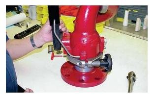
Align 'hexes' and push valve handle onto trunnion while engaging slide link in hole on bell.
