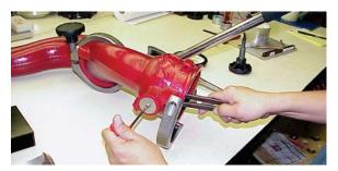
7) Using the T-handle hex wrench, remove washer, plug and screw. These parts are not reused with the valve parts.
