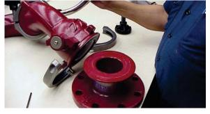
3) Open the Clamps and lift the top of the Protector off of the Flanged Base.
