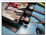
4. Feed the crimped ends of the cable through the strain relief fitting.
