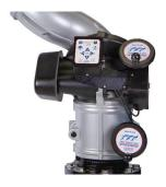
Choose between manual or remote control (RC) version 12-24 VDC. All models have easy to rotate dual hand wheels. Operate from a distance by remote control using a wide selection of wired. wireless, and CAN options. Customize your operating envelope with field changeable rotation stops
