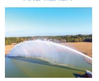
An integral stream straightener and only 15 psi (1.0 bar) friction loss at 8000 gpm (30,000 l/ min) gives the lowest turbulence and the greatest reach; up to 400 ft (120 m) horizontal or 210 ft (64 m) vertical distance in still wind conditions.
