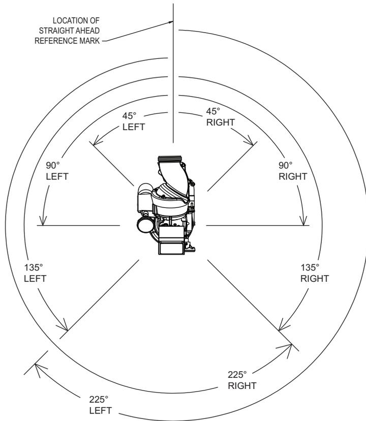
**RC MODELS WITH NO TRAVEL STOPS INSTALLED HAVE A HORIZONTAL ROTATIONAL TRAVEL LIMIT OF 225° LEFT AND RIGHT OF THE STRAIGHT AHEAD REFERENCE MARK**
