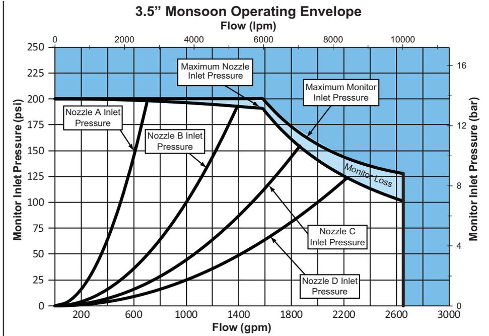
Nozzle A flows 500 gpm (1900 l/min), at 100 psi (6 bar), K factor = 50
