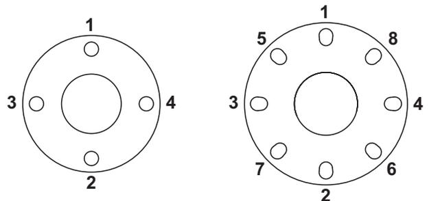
Tighten Sequentially Each Bolt Three Times
