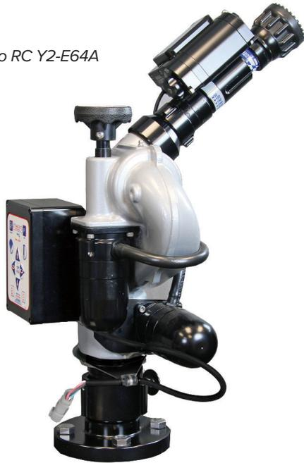
The TORNADO® monitor series is available in a manual or RC version. Models are compact, yet capable of flowing up to 500 gpm (1900 l/min). They are an ideal bumper turret and have a 370° horizontal rotational or 180° with user installed travel-limit stops. The elevation range is 90° above horizontal to 45° below. Discharge elbows include an integrated stream straightener. An RC LT version is also available for lower profile applications.
