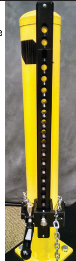
Install Backbone in 1st Chain Block
