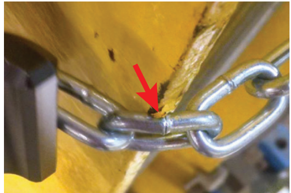
Figure 4.9.1.1 Chain Bending Against a Sharp Corner
