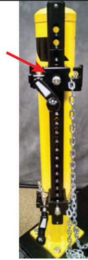
Install 2nd Chain Block on Backbone
