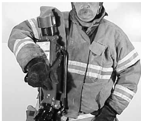
Figure 5.2 Carrying the Blitzfire on an Uncharged Hose
