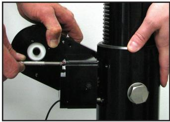
Verify that the tube latches in the fully extended and fully retracted positions and not in any intermittent positions. If intermittent latching occurs, remove the gearbox and check the orientation of the timing marks.
