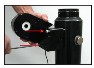
4 Ensure that the timing marks are in the correct orientation. This may take several knob rotations.
