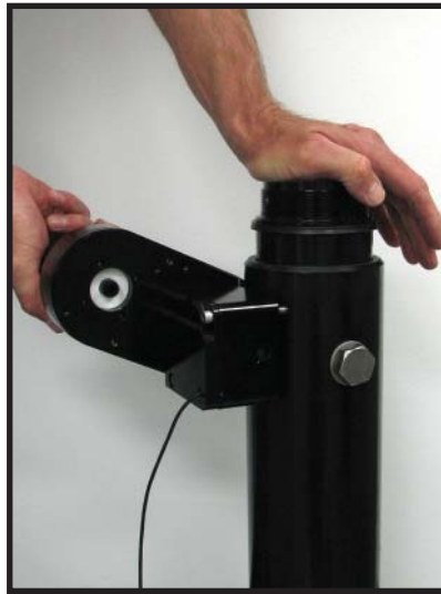
To release down latch, push down on tube while turning knob.
