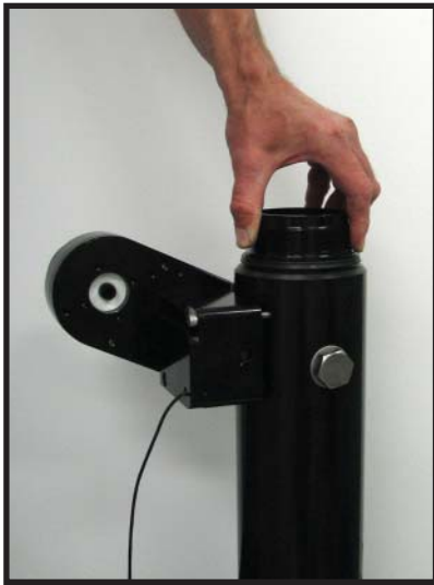
To test down latch, pull up on tube while in down position.
