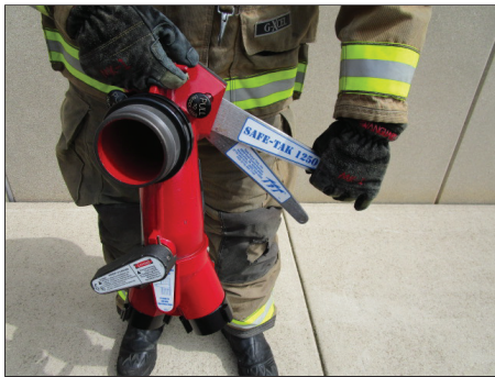
Grasp and pull up on the longer leg until the lock engages.
