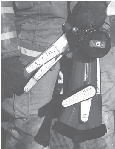
Figure 4.2.1 Hold base carrying handle and grasp end of longer leg
