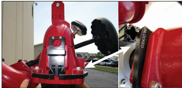
Slide Bar in the UP position. Plunger and pawls UNLOCKED.
