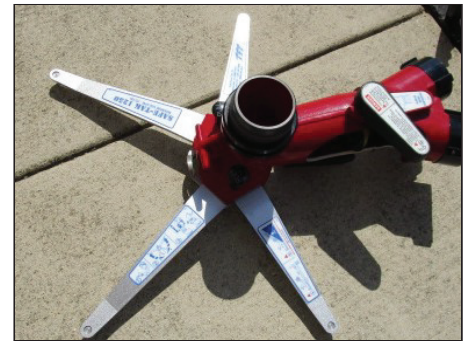
Place the base on the ground with all spikes making contact. Remove the cap and anchor strap for later use.
