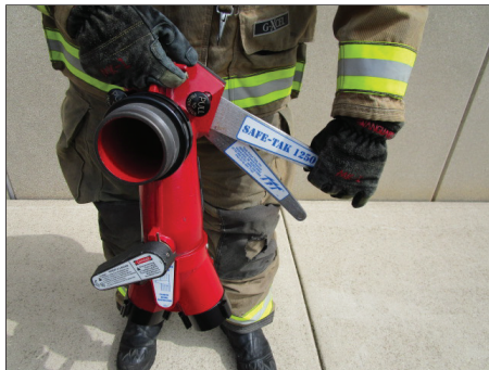
Grasp and pull up on the longer leg until the lock engages.
