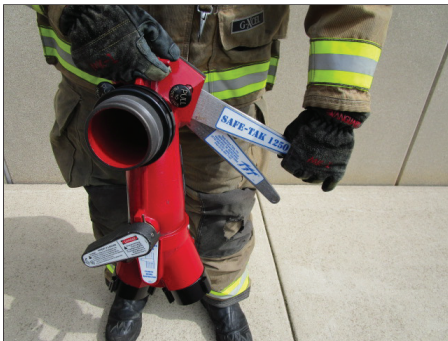
Grasp and pull up on the longer leg until the lock engages.
