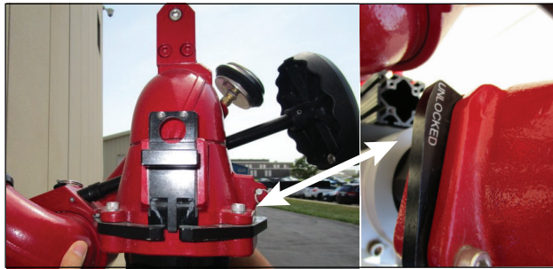
Slide Bar in the UP position. Plunger and pawls UNLOCKED.
