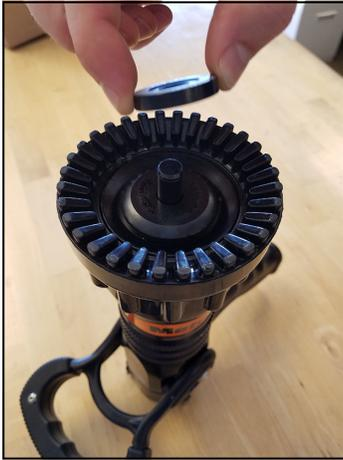
**STEP 4** - Remove the old flow calibration disc from the shaft, leaving the baffle installed.
