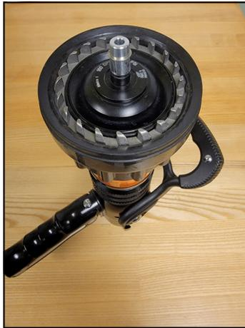
**STEP 6** - Place a **NEW** Spirolox ring over the installation cone.
