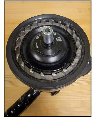
**STEP 5** - Place the new flow calibration disc over the end of the shaft, followed by the metal installation cone.
