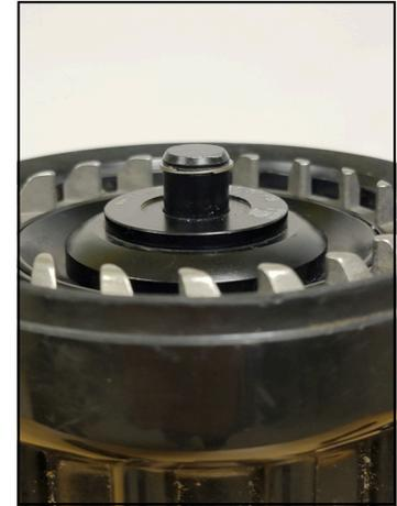
**STEP 8** - Visually verify Spirolox ring is fully seated in the groove. Move the shaper to straight stream and flow test the nozzle.
