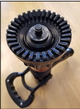
**STEP 1** - Set nozzle to the flush position. Push the baffle and flow calibration disc down to expose the Spirolox® retaining ring.
