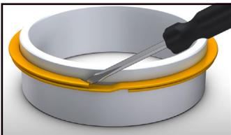
Pry the end of the ring out of the groove and up.
