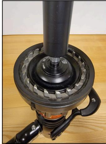
**STEP 7** - Place the pusher tool over the cone and press down to install the ring in the groove in the end of the shaft.
