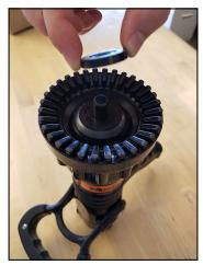
STEP 4 - Remove the old flow calibration disc from the shaft, leaving the baffle installed.
