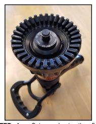
**STEP 1 -** Set nozzle to the flush position. Push the baffle and flow calibration disc down to expose the Spirolox® retaining ring.
