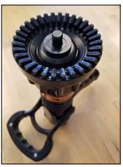
**STEP 3 -** Pull ring out of the groove by unwinding in a clockwise direction. **DISCARD THE RING.** Use care to avoid deforming the groove in the shaft.
