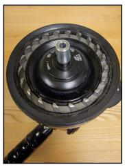
STEP 5 - Place the new flow calibration disc over the end of the shaft, followed by the metal installation cone.
