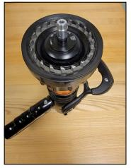
STEP 6 - Place a NEW Spirolox ring over the installation cone.
