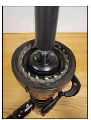
STEP 7 - Place the pusher tool over the cone and press down to install the ring in the groove in the end of the shaft. **ALWAYS USE A NEW SPIROLOX**
