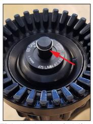
**STEP 2 -** Use the point of a knife, pick, or small screwdriver to pry the end of the retaining ring out of its groove.
