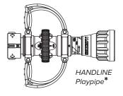
The 2.5" HANDLINE features flush without shutting down, patented slide-type valve for turbulence-free flow control, six detent flow positions, molded rubber teeth for full-fill "power fog," and "Gasket Grabber" inlet screen. They utilize lightweight hard coat anodized aluminum materials for maximum resistance to corrosion and wear. 2.5" NH (64mm) rocker lug swivel couplings are standard. Folding pistol grips and NFPA color handles and grips are also available.
