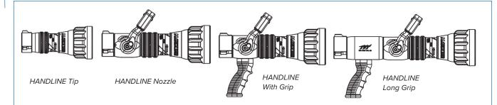
The 1.5" HANDLINE features flush without shutting down, patented slide-type valve for turbulence-free flow control, six detent flow positions, molded rubber teeth for full-fill "power fog", and "Gasket Grabber" inlet screen. They utilize lightweight hard coat anodized aluminum materials for maximum resistance to corrosion and wear. 1.5" NH (38mm) rocker lug swivel couplings are standard. Folding pistol grips and NFPA color handles and grips are also available.
