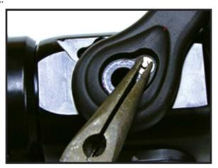
**Step 3)** Holding your thumbs over the detent balls and springs on the bail handle pull the handle upward and off using your thumbs to capture the balls and springs when the handle is removed.
