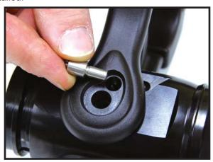
**STEP 7)** Apply red Loctite® to the threads of the button head screws that retain the handle. Install one on each side of the handle until hand tight.
