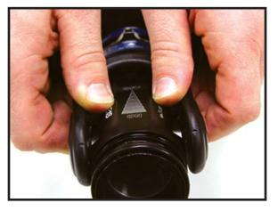
**Step 4)** Align the cam pin hole in the valve disc with the groove in the slider. Insure that the cam pin hole is facing up nearest the valve detent arc.
