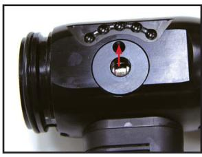
**Step 5)** Install the detent springs and balls into the bail handle. Using the same method as when the handle was removed retain the springs and balls in the handle with your thumbs. Install the handle over the valve snapping it into place. Insure that the valve handle is oriented as indicated in the photo. The cam pin hole should be forward toward the exit of the nozzle.
