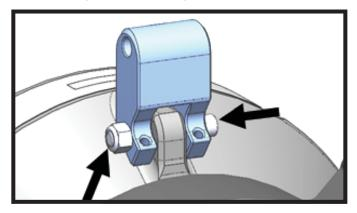
**2**. Apply blue Loctite to 3 threaded holes in Hinge Block. Tighten 3 Set Screws until heads are flush with Block.
