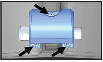
**3.** Hold wallet-size card against Hinge Block and Strainer. Pull upwards on Hinge Block and tighten Set Screw nearest to card until it bottoms out, then remove card.
