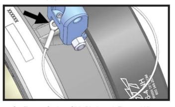
**6**. Set Float on Strainer. Slide Pin through Float and Hinge Block, then latch the Pin.
