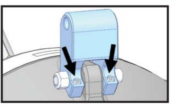
**5.** Set Cable eyelet against vertical Set Screw. Loosen Screw until eyelet slips under it, then tighten Screw through eyelet until snug against Strainer.
