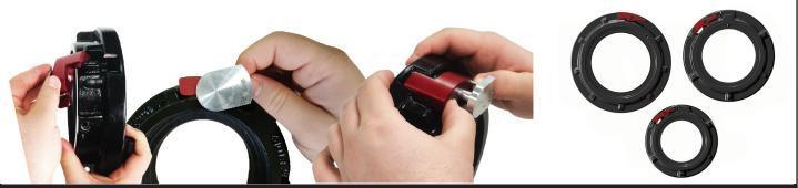
STEP 3 - Align the storz tool with the cylindrical post on the storz coupling. While holding the coupling use both thumbs to press lever until it is fully seated. Operate the lock several times to insure free movement.
