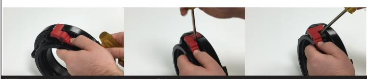
STEP 1 - Use a large flat screwdriver to push the lever off it's post while maintaining the lever in the down position
