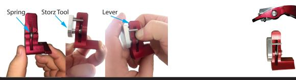
STEP 2 - Insert spring into either the: 4", 5", or 6" aluminum lever with the small ear of the spring facing forward flat against the surface. Line up spring and lever holes before inserting THA403 tool partially. Fold large ear in and fully seat lever against tool insuring the long ear is captured under the dowel pins of the tool.
