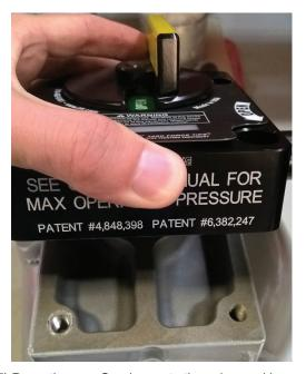
**STEP 5)** Press the new Gearbox onto the valve, making sure to align the Trunnion on the Gearbox to the Trunnion hole on the Valve Ball. Some adjustment of the Valve Ball may be needed in order to properly align the Gearbox Trunnion with the mating socket of the Valve Ball.
