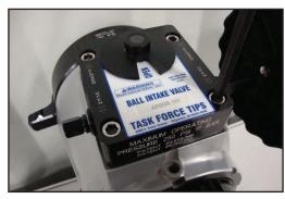
STEP 1) Place the ball valve into the full open position. Using the 5/16" Allen wrench, remove the socket head cap screws that retain the existing gearbox assembly to the valve body.
