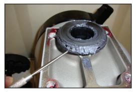
STEP 2) Using the seal pick, carefully remove the Gear Spacer STEP 3) Visually inspect the O-ring that is in the valve body. that is pressed into the top of the valve body.
