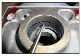
Verify that it is not worn or damaged. Replace with 128 O-ring if necessary.
