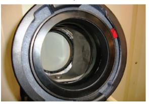
STEP 4) Place the Valve Ball and the new Gearbox in the open position. Viewed from the inlet or hose side of the valve, the Valve Ball should be rotated to the right or 3 o'clock position. If ball is difficult to rotate, lightly apply grease to the lower trunnion and mating hole in the half Valve Ball.
