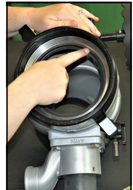
5. Run the pointed end of the seal pick around the outer edge of the seat to ensure that the seat is not hung up on the edge of the threads.
