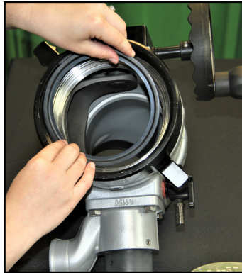
4. Install a new VALVE SEAT into the BACK RING with the lip on the seat toward the VALVE BALL.
