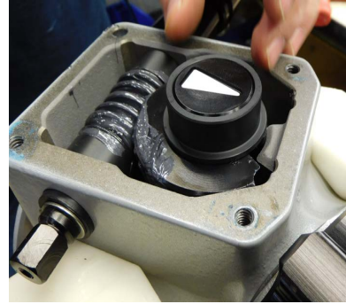
18. Reinstall the bearing over the gear.
