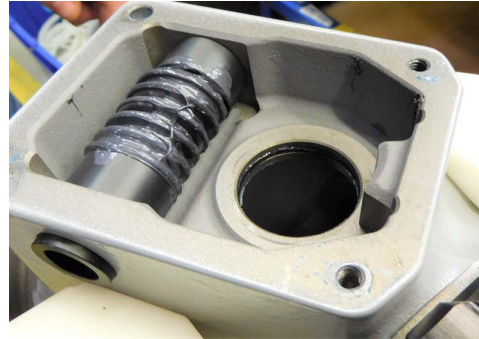
12. Install a new VO-128 and apply Molykote #112 High Performance Silicone Grease over.
