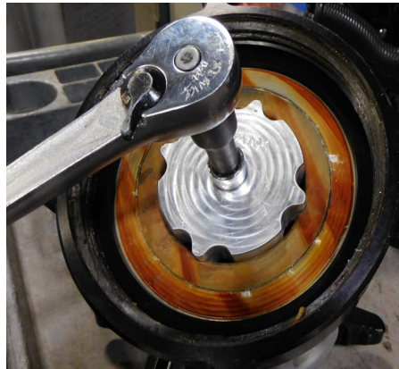
7. Use THA409 to screw the SEAL RETAINER into the BACK RING to 1/16" below flush.
