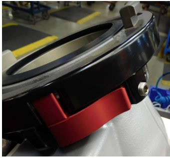
1. Use a hex key to remove the LOCKOUT SCREW from the Coupling.
