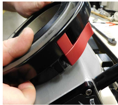
6. Firmly press the coupling onto the Valve Body. Verify the seal is not protruding from the joint.
