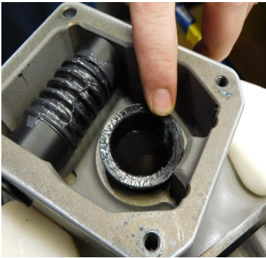
13. Reinstall the bearing.
