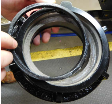
3. Remove the CUP SEAL from the Storz Coupling.
