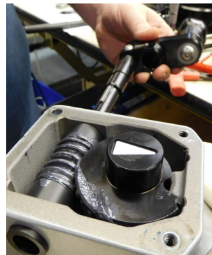
16. Insert the shaft through the worm gear. The key in the shaft will engage the slot inside the gear.
