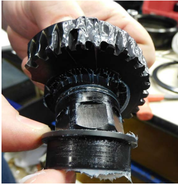
9. Remove the bearing from the gear.
