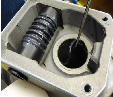
11. Use a seal pick to remove the VO-128 O-ring from the casting.
