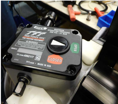
19. Place the cover on the gear box.
