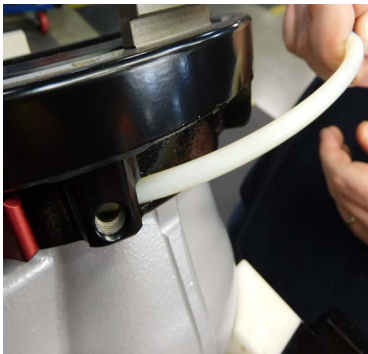
7. Push the BEARING STRIP back into the groove, blunt end first. Rotate the coupling to help pull the strip in.
