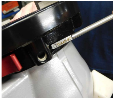
2. THA401-ST to hook the end of the BEARING STRIP. Pull the strip out of the groove.
