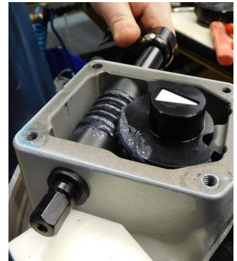
16. Insert the shaft through the worm gear. The key in the shaft will engage the slot inside the gear.
