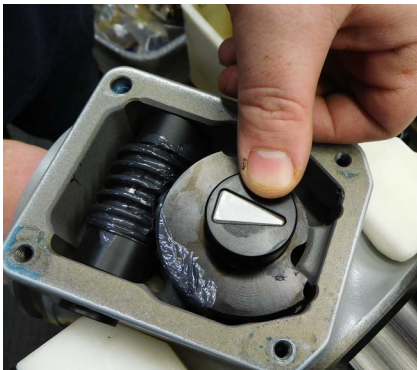
15. Firmly reinstall the gear with the arrow pointing away from the meshed gear teeth.
