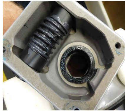
14. With the ball in the open position (top side of valve, not blocking the waterway or PRV), align the side having the hex with the hole in the gear box.
