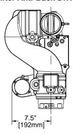
If the amount of clearance required for the anti-back-drive gearbox is not available there is also an electronic method to help prevent unintended monitor/nozzle movement due to vibration. The electronic method can only be used if the monitor is always powered while the truck is in operation. See LIY-500 Section 4.13.3 for wiring and programming information. If the anti-back-drive gearbox upgrade (Y4917-KIT) is purchased separately, see LIY-203 for installation Instructions.
