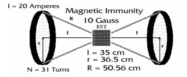
Calculate: Field Strength (V/m) at point halfway between the coils.
