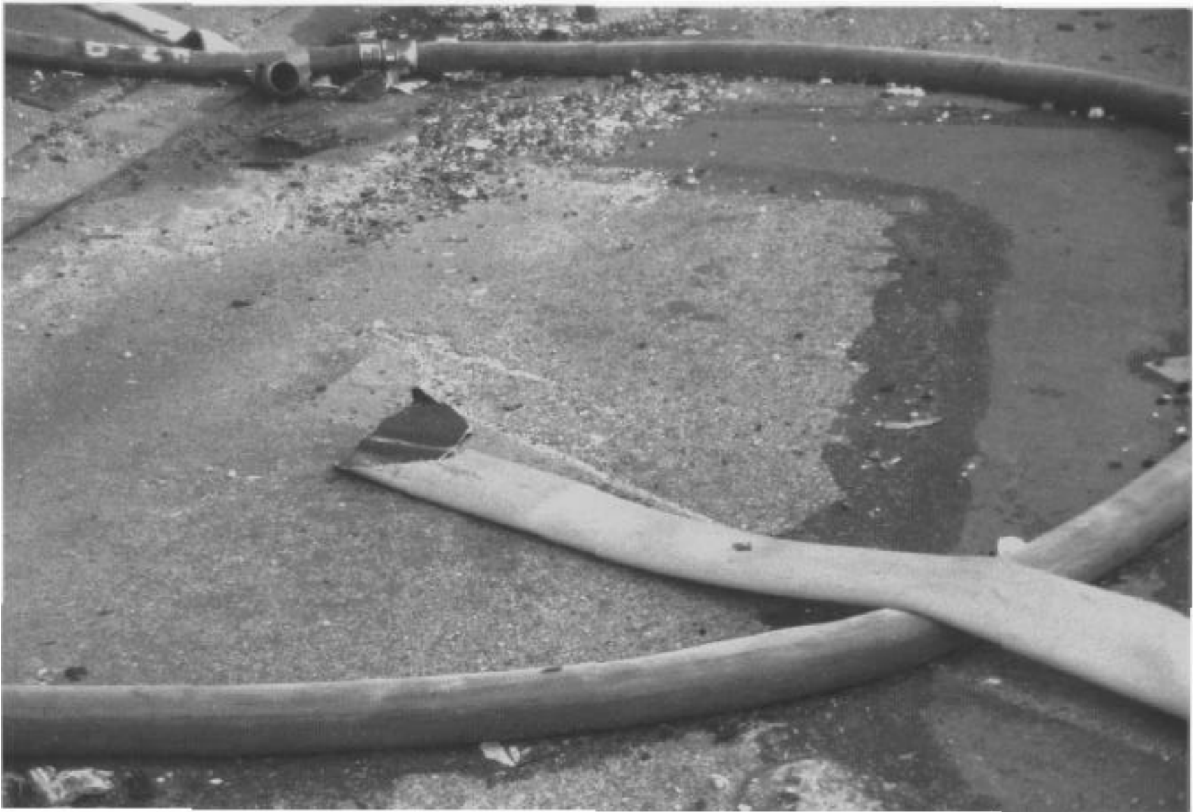
Section of 5-inch hose that was ruptured by falling debris outside the building. Hose lines feeding the standpipes and entering the stairways were damaged several times and had to be replaced at great risk to firefighters. (Shoring boards were later used to protect the hose lines.)
