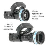
With a retracted sleeve, the nozzle operates as a standard dual gallonage straight stream/combination nozzle. To use the nozzle's aspirating feature, simply slide the outer sleeve forward. If an immediate wide fog pattern is needed, the sleeve can be retracted instantly to its regular position.
